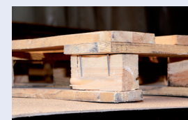
Visible fastening elements e.g. nails
